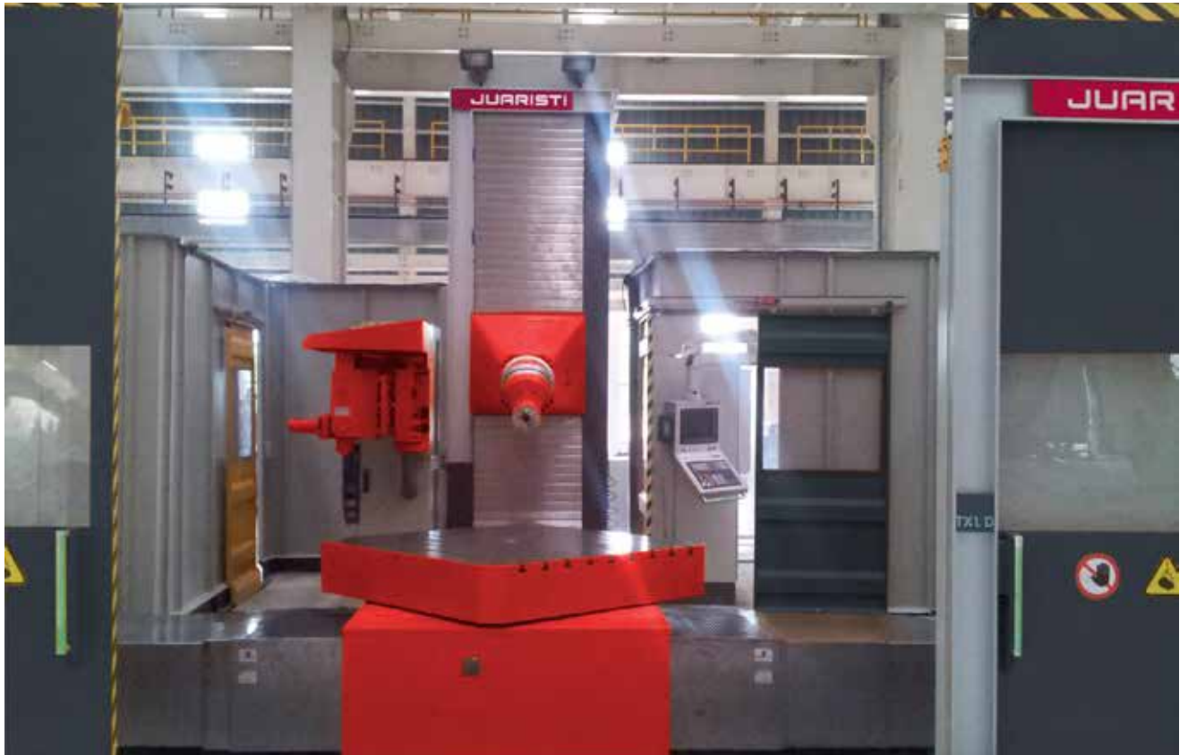
TX1 model with 37 kW Automatic Universal Head
