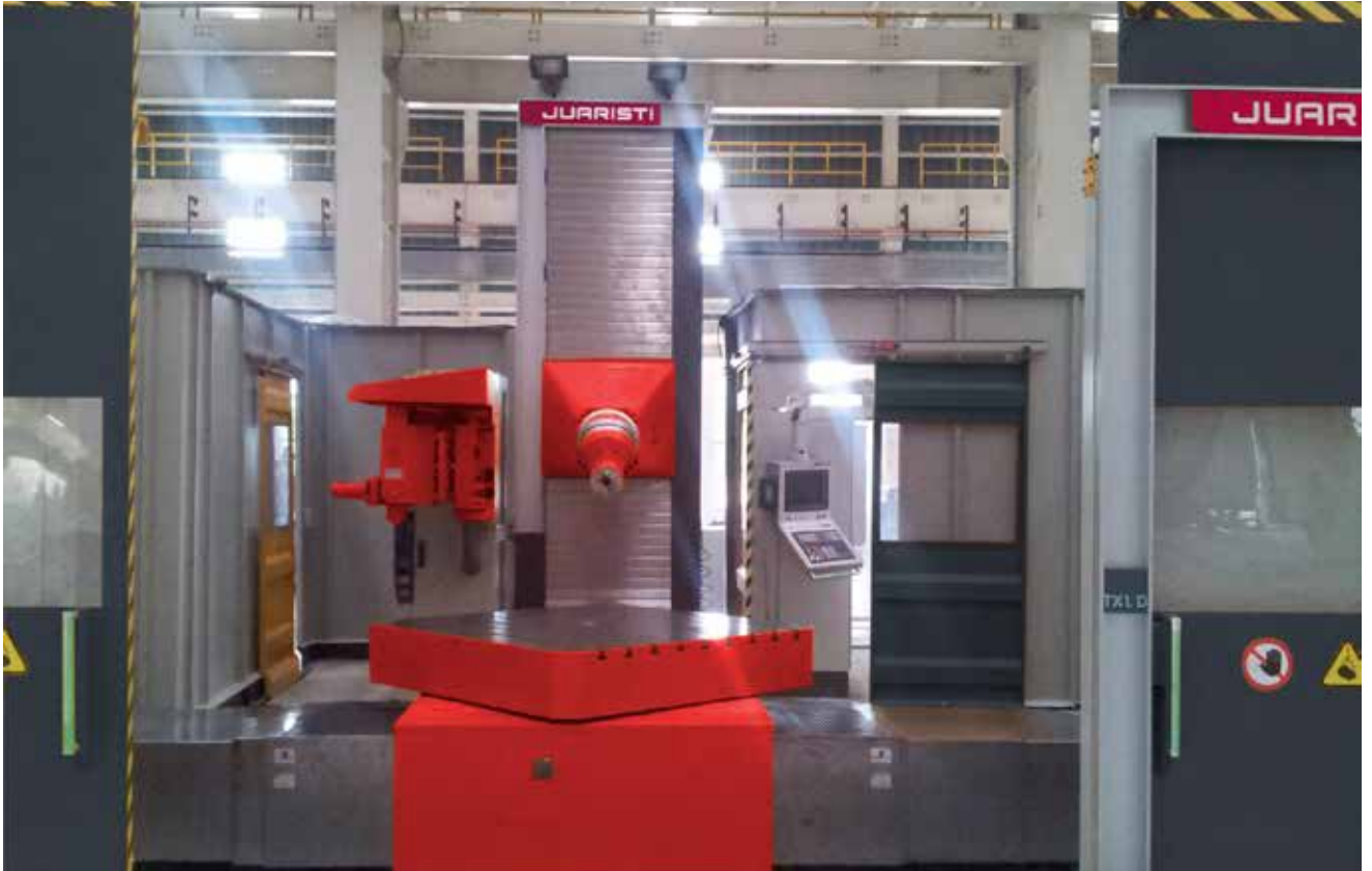
TX1 model with 37 kW Automatic Universal Head
