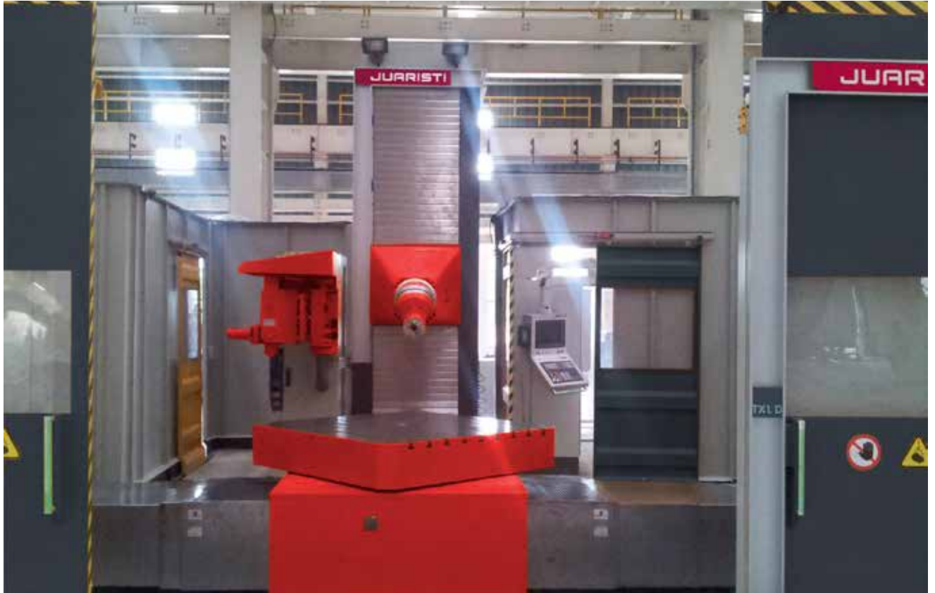
TX1 model with 37 kW Automatic Universal Head
